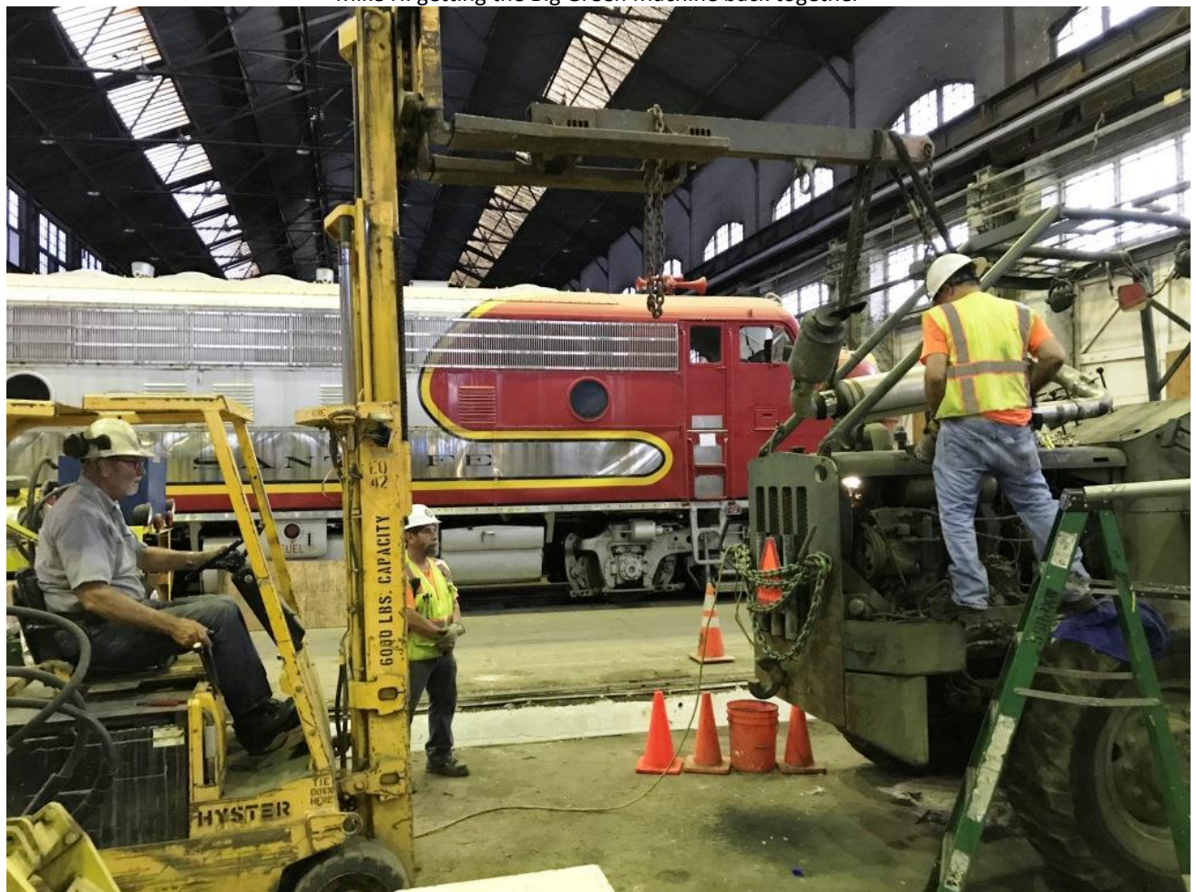
Alan uses the forklift with the stinger attachment to lift the exhaust system back onto the Big Green Machine
