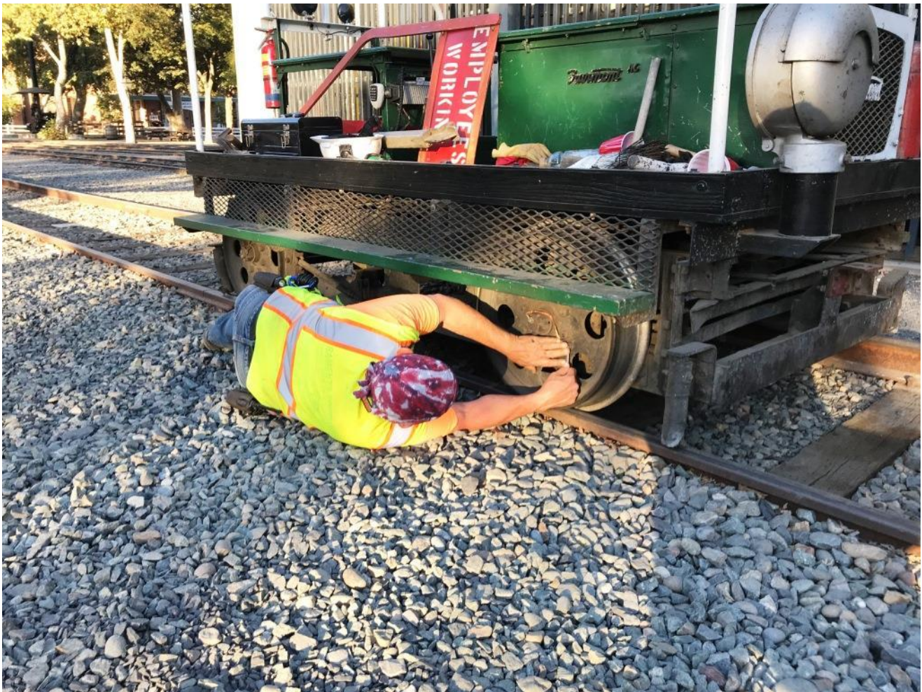
Don't worry. Joe's just fine. He's just fixing the shunting wire on the motorcar's wheel and axel
