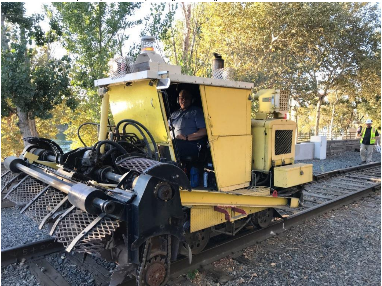
Chris moves the scarifier onto the 150 Track
